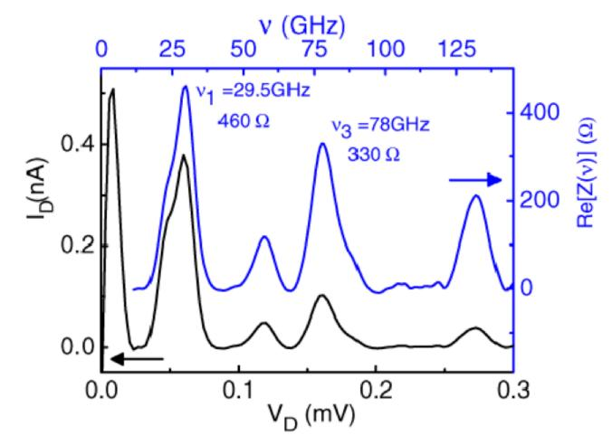
$I(V) = \operatorname{Re}[Z(2eV/h)]I_C^2/2V$   $Z(\omega) - \text{ impedance of the resonator}$  $I_C - \text{ critical current across the junction}$
